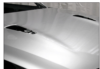
Figure 8– Nissan color code KAB is a four-stage refinishing color from the vehicle maker.
