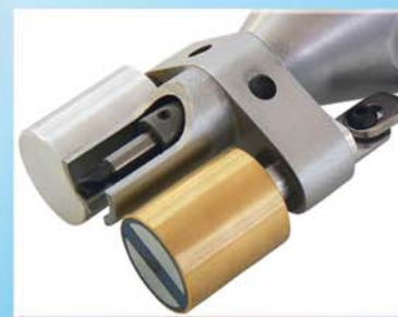
Centrally mounted chuck for the special drill bits with good visibility
