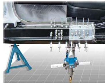
Magnetic support system with a capacity of 2 x 35 kg
